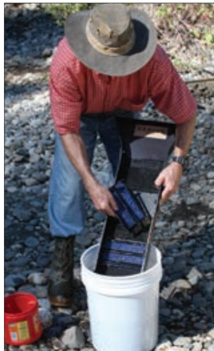
Plastic riffles and "miner's moss" are removed from the E-Z Sluice as part of the cleanup process.
