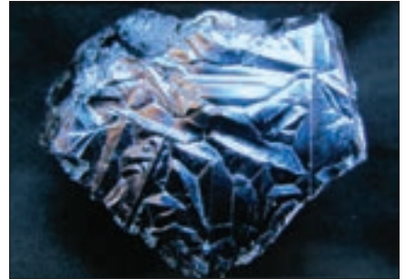
Elemental silicon, which is rarely seen, has a bright metallic luster and an attractive blue iridescence.
