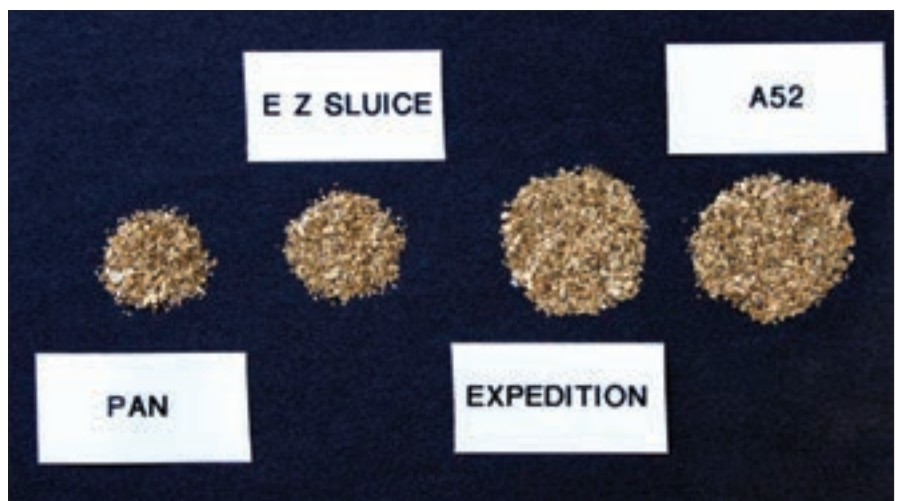
Nearly all the gold captured by the sluices and pan was minus 20 mesh and smaller, which means this exercise was an excellent test of their abilities to capture fine gold.
