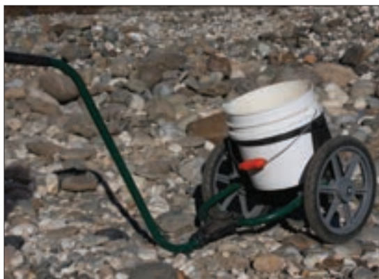
The Broll hauler holds a 3- or 5-gallon bucket and makes it easier to move a bucketful of rock to the river for sluicing.
