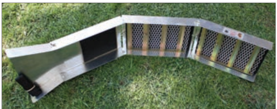
The flair on the Jobe sluice is removable and the entire box can be folded into a small package for backpacking.
